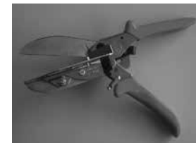
Demultiplied mitre shears Reference: Janser: 262 284 000. For cutting around door frame bases, areas which are difficult to access.
